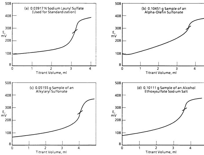
FIG. 1 Potentiometric Titration Curves of Various Anionic Surfactants versus 0.03757 N Hyamine 1622 Using the Orion Model 93-07 Nitrate ISE
